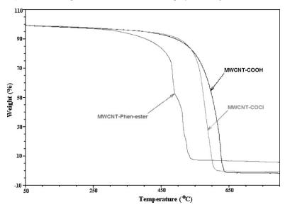
**Figure 5.**Thermal degradation in an air atmosphere of functionalized MWCNT-carboxyl through ester-linked phenanthroline.
