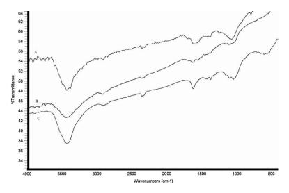
**Figure 7.**Infrared spectra of carboxy-functionalized MWCNT (MWCNT-COOH, A), the corresponding acid chloride (MWCNT-COCI, B), and ester-linked phenanthroline-MWCNT (MWCNT-Phen-ester, C).
