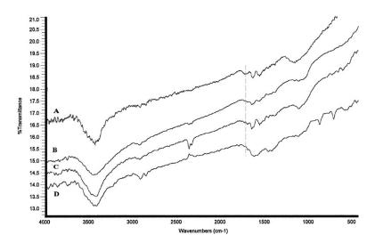
**Figure 4.**Infrared spectra of functionalized MWCNT-carboxyl through ether-linked phenanthroline. MWCNT-COOH (A), MWCNT-CH2OH (B), MWCNT-CH2OTS (C), MWCNT-Phen-ether (D).
