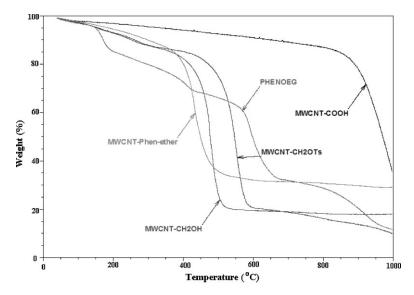
Thermal degradation in a nitrogen atmosphere of functionalized MWCNT-carboxyl through ether-linked phenanthroline.
